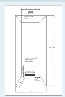
\*The given cabinet opening height dimension includes space for top air vent. If you choose to place the vent above the cabinet or in a soffit, you will need to adjust the height dimensions accordingly. Please refer to Ventilation
