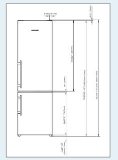
When installing CS units into a row of cabinets or wall units: Use these dimensions to achieve a custom look with the cabinetry while providing the necessary clearance for the top door hinge.
