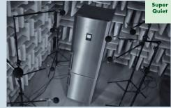
SuperQuiet: Noise is kept to a minimum with virtually silent, speed controlled compressors and a low-noise cooling circuit; while also ensuring exact performance, energy efficiency and SuperQuiet operation.
