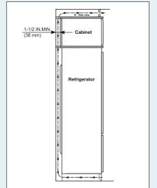
This type of cabinet must be carefully constructed using the correct dimensions and it must provide suitable ventilation to ensure proper appliance operation.
